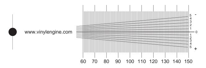
Check that the distance beetwen the line passing through the black circle and the 150 line is exactly 150mm
